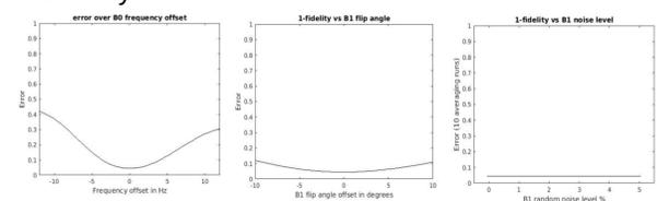
Left: B0 frequency offset versus error. Middle: B1 flip-angle offset versus error. Right: B1 white noise level vs error order 10 averaging runs.
