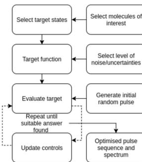
Figure 4 : Program flow, optimisation loop terminates when convergence falls below a tolerance level.
