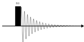
Figure 3 : A basic free induction decay (FID) pulse sequence, a 90° excitation pulse followed by a readout [2].
