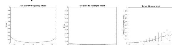
Left: B0 frequency offset versus error. Middle: B1 flip-angle offset versus error. Right: B1 white noise level vs error order 10 averaging runs. Error is (1-fidelity), where an error of 0 would represent a perfect match between target state and actual state produced by the pulse sequence. A flatter landscape represents a more stable pulse.
