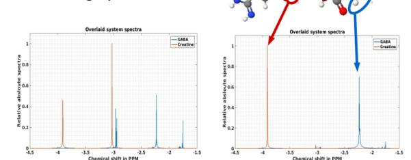
Above: Comparison of a 90° excitation pulse (left) and an optimised pulse (right). Optimised pulse is stable to 10Hz B0, 10° flip angle T=3ms.
