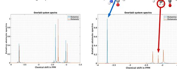
Above: Comparison of a 90° excitation pulse (left) and an optimised pulse(right). Optimised pulse is stable to 10Hz B0, 10° flip angle T=222ms.
