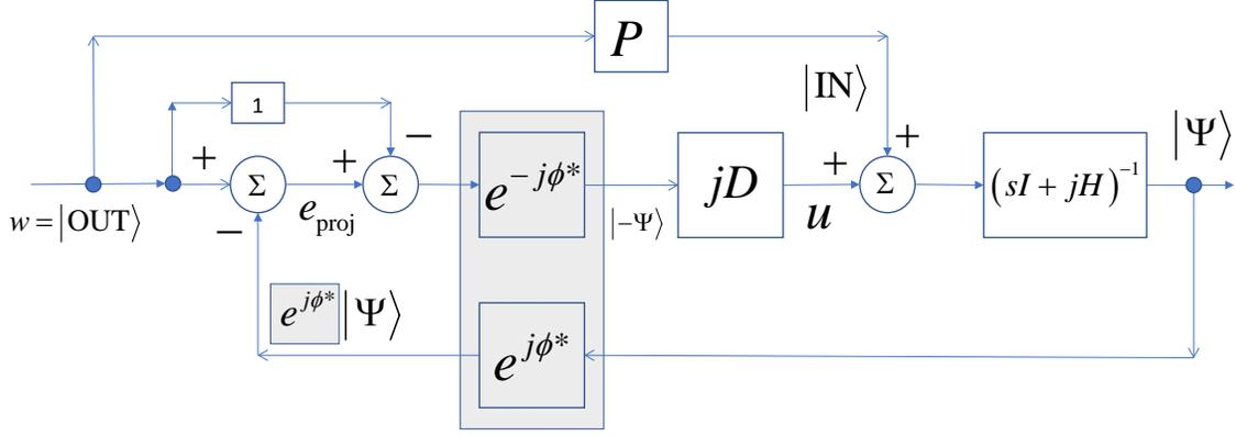
Fig. 2: The projective error  $e_{\text{proj}}$  embedded in a semi-classical 3-degree-of-freedom loop. The top paths ( $P$  and  $1$ ) are indeed two additional degrees of freedom relative to the single degree of freedom configuration. The shaded areas refer to the “global phase factor.” Note that the  $e^{\pm j\phi^*}$  operations have to be interpreted in the time-domain.
